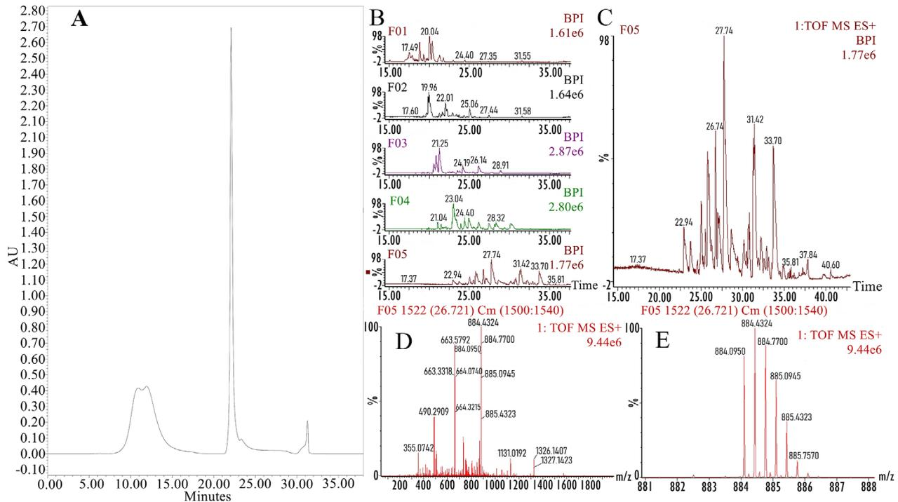
**FIGURE 2** (A) Representative chromatogram of one depletion run. The first peak represents the low abundance proteins and the second peak represents the high abundance proteins or the depletome. (B) Five representative chromatograms of 2-D LC fractionation before MSE analysis. (C) Zoom in on the last chromatogram of figure 2B, related to fraction 5 from that run. (D) Representative spectrum corresponding to data acquisition at the peak at 26.74 of fraction 5. (E) Zoom in on spectrum shown in D
